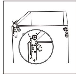
7. Unscrew right middle stopper with metal block from bottom of upper door. And then install left middle stopper and metal block in left side of bottom of upper door. (The same operation as for lower door.)
