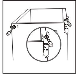
5. Unscrew and remove the bottom hinge pin, turn the bracket over and replace it.
