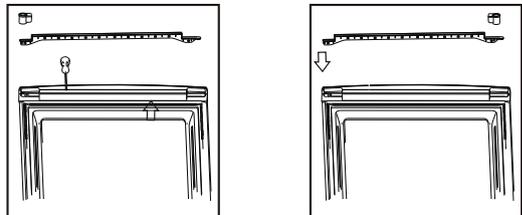
3. Unscrew from the middle hinge by cross screwdriver, then take off the lower door.
