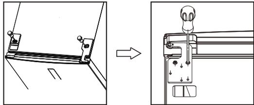
2. Please upwarp and take off plastic cover and wire sleeve by straight screwdriver. Please be careful of the wire inside. Then move wire with connector to another side and install wire sleeve to another side and fix cover back.
