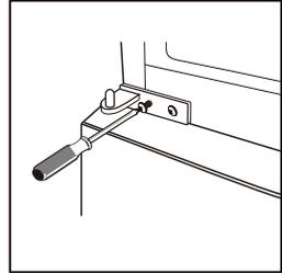
9. Install the upper door, fix the upper door hinge onto the cabinet and connect the wire.
