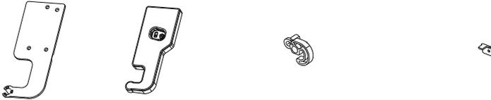
1. Close upper door, take out the screw from the top hinge covers by cross screwdriver. Take off hinge cover, disconnect the terminal, then unscrew top hinge and take off upper door.
